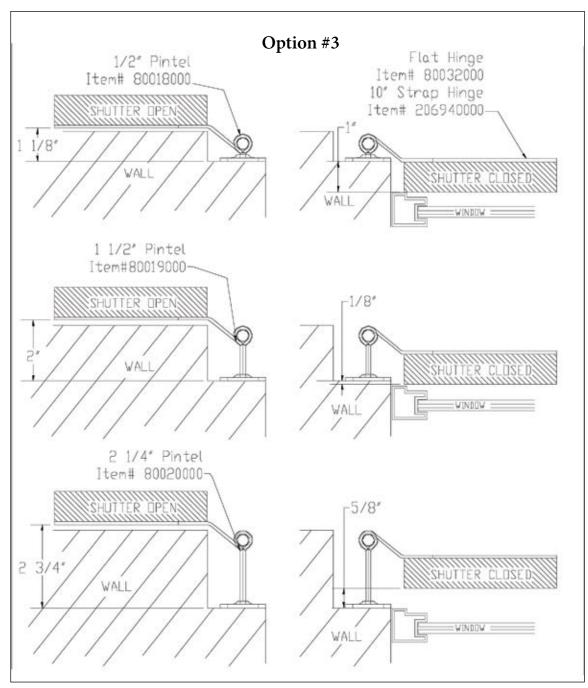
The ideal setup is to have the Shutter flush with the casement when the Shutter is in the closed position. The Pintel Shims can be added to make small adjustments of 1/4", 1/2" and 3/4".
