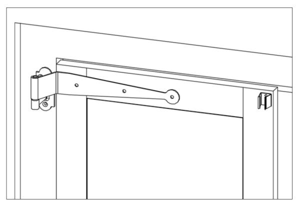
Swing the shutter open and mark the location for the Acorn Clip on the wall. If mounting in a wood surface drill a 1/4" pilot hole and mount the Acorn Clip. If mounting in a masonry surface use the appropriate anchor.
